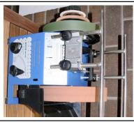
Figure 2: frontal vertical base applied to the grinder
